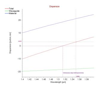
In this example, we will modify the fiber design to obtain zero dispersion at the selected wavelength of 1.55  $\mu$ m. From the dispersion calculation, we see this design has a dispersion of about 3 ps/km/nm at the selected wavelength.
