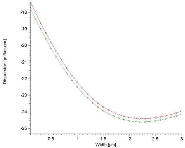
From this graph, we see that in order to shift the dispersion by 3 ps/km/nm, the width will need to be increased to some value between 1.3 and 1.4 μm.
