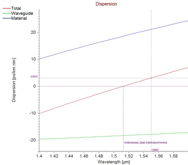
In this example, we will modify the fiber design to obtain zero dispersion at the selected wavelength of 1.55 μm. From the dispersion calculation, we see this design has a dispersion of about 3 ps/km/nm at the selected wavelength.
