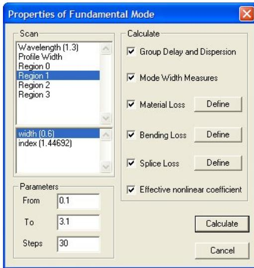
Here the width of Region 1, the layer between the core and the outer ring, is varied from 0.1 to 3.1.
